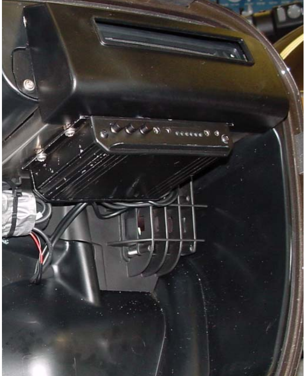
BC VOICE installed position / Cooling Fan
