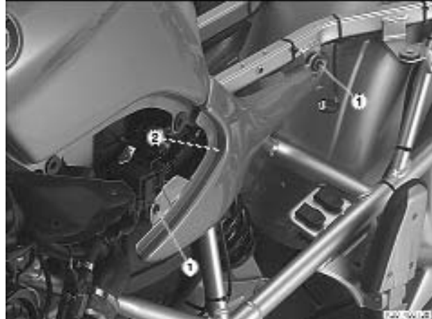
Remove Left and Right side covers
