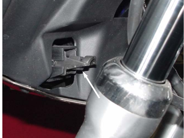
Base setting adjustment screw
