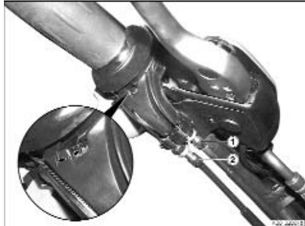
Cable Adjustment Points
