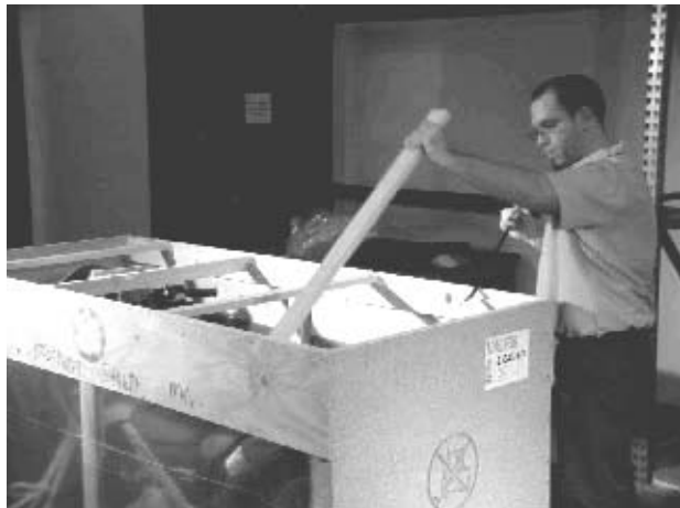
Carefully lever out top supports
